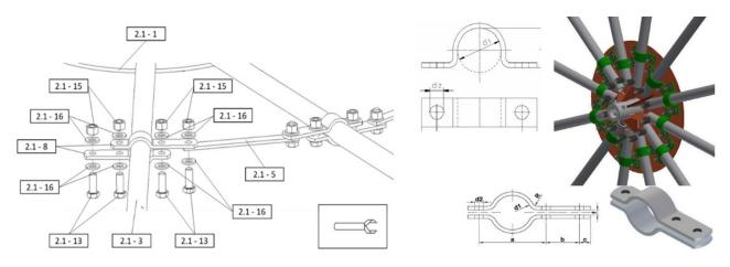
You can also easily build the ring that accurately positions the rotor blades with asymmetrical pipe clamps. We are looking forward to your experience reports, especially if you build a rotor with a different diameter.
