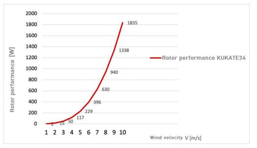
It has a coefficient of power of 0.35. The coefficient of performance is so high because we in the area calculation the inner "pane" is not taken into account.
