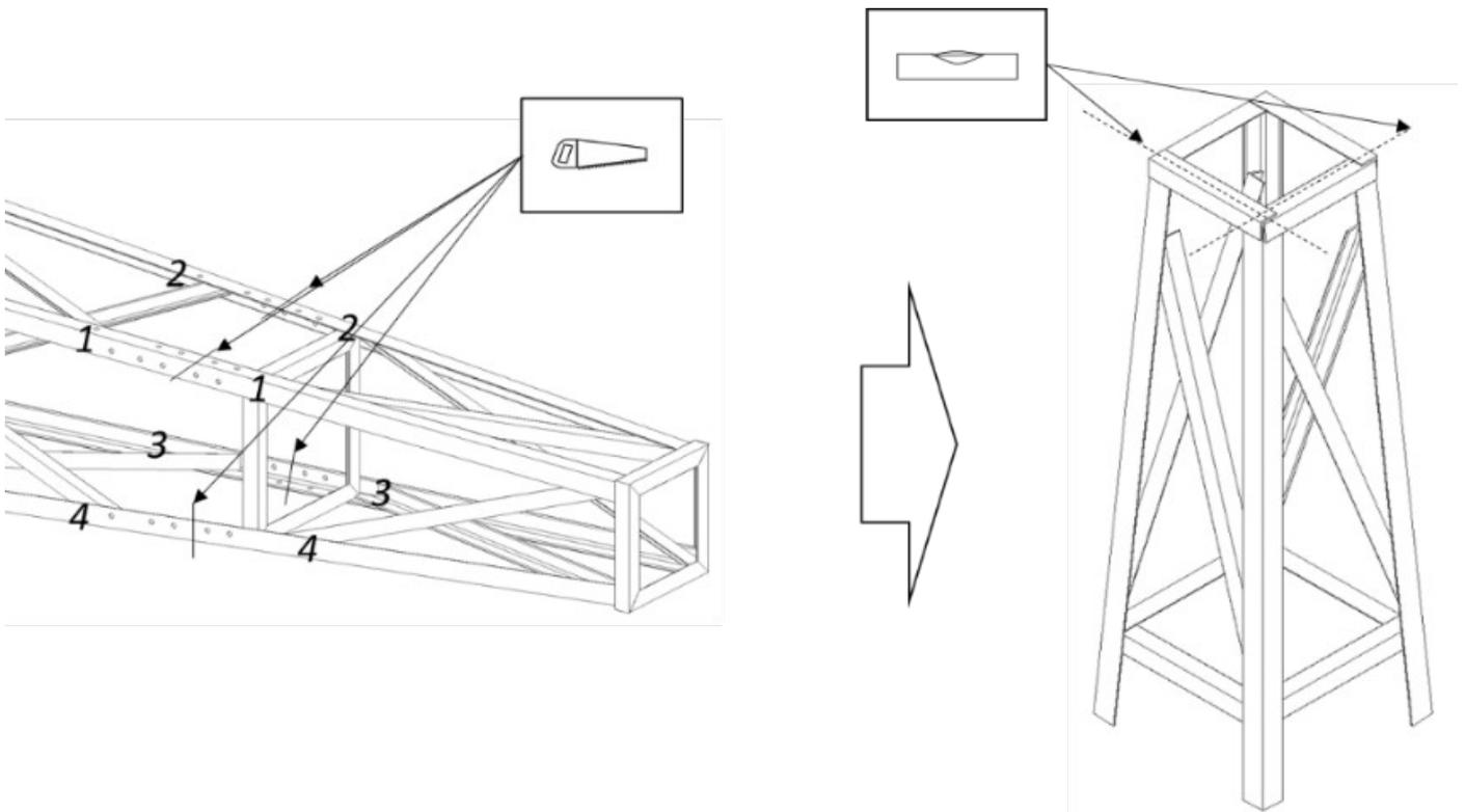
3. **Position the head plate very accurately and weld it in place**
