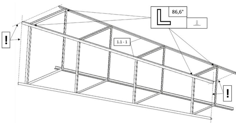
6. In the next step, the other two longitudinal struts are placed and dotted. Here, it is also very important to ensure that **the angle and distances of the longitudinal struts to each other and to the cross strut squares are maintained**. This must be done with particular care, otherwise the mast will not be straight.
