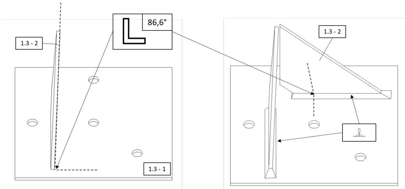
3. Next, the two mast bases with the hinges are fabricated. To do this, weld the plates [1.3-5] at right angles (90°) to the outer edge of the base plate [1.3-3]. Then the tubes [1.3-7] are placed and welded. Make sure that the center lines of the holes are aligned **exactly**.
