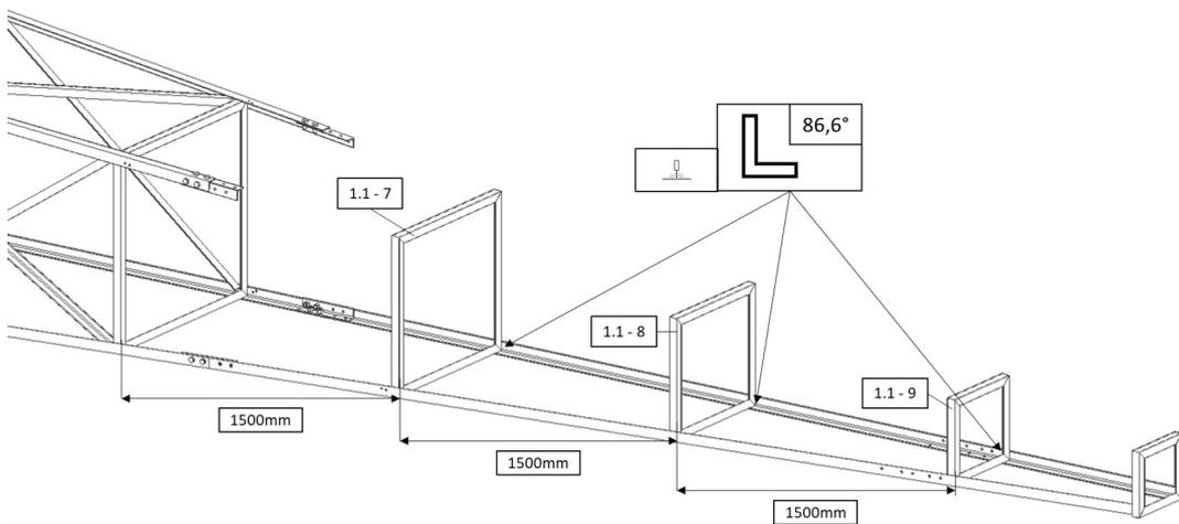
9. Keeping the angles 3.4 degrees and 86.6 degrees, respectively, the middle crossbar squares [1.1-7], [1.1-8] and [1.1-9] can now be positioned, aligned and punctured.
