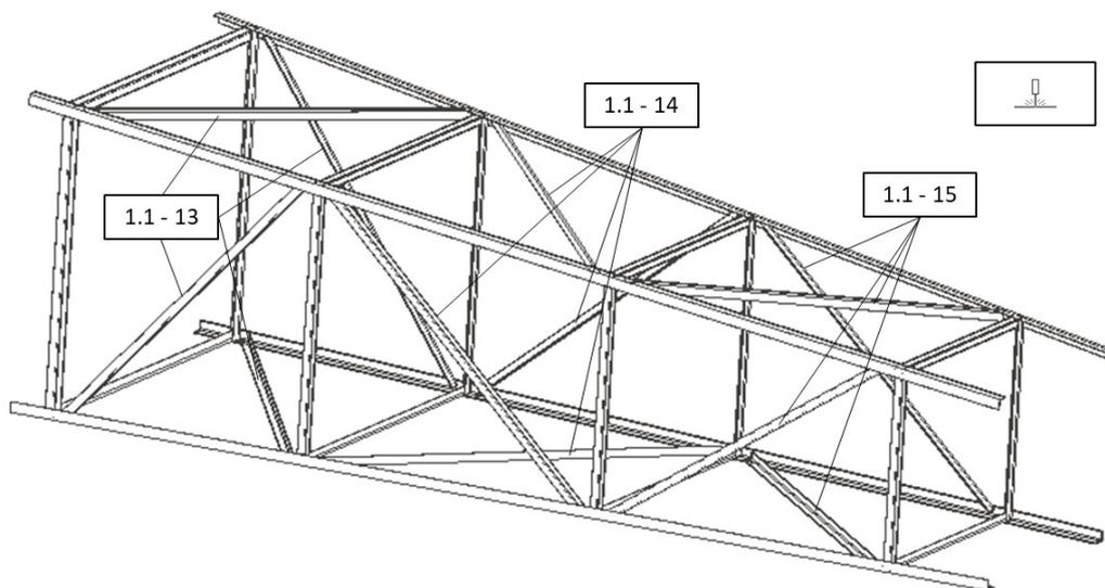
8. **Build upper half of the mast and connect it with the lower one**
