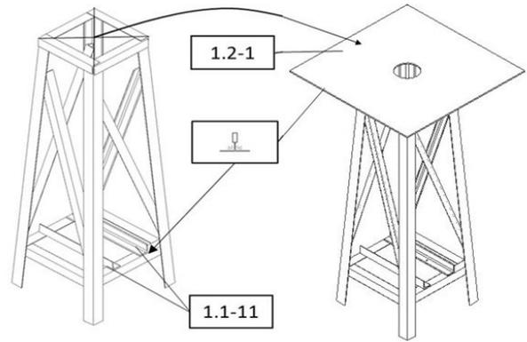
The upper steel plate [1.2-1] must be aligned **exactly parallel** in the plane of the mast feet at the bottom. The tube must be **exactly vertical** on the plate!
