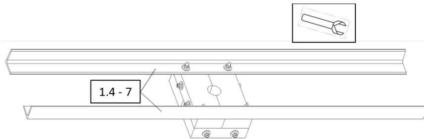
3. The bearing 3 is screwed to the matching holes of the L-sections [1.4-7].
