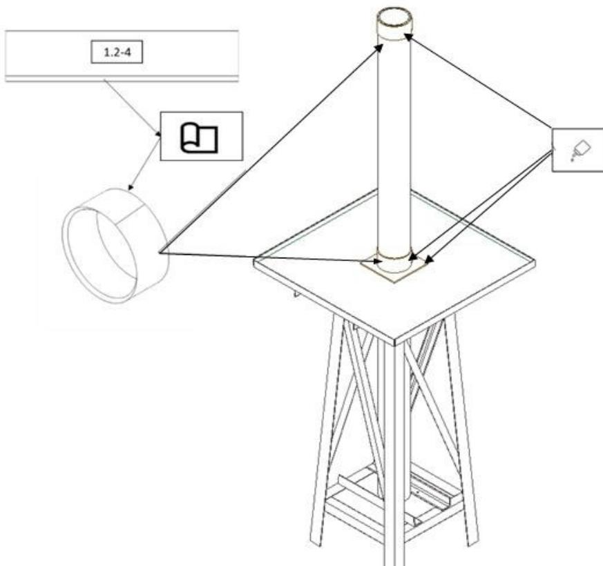
Only when everything fits exactly are the bearing sleeves glued to the top and bottom of the mast tube with a suitable adhesive.
