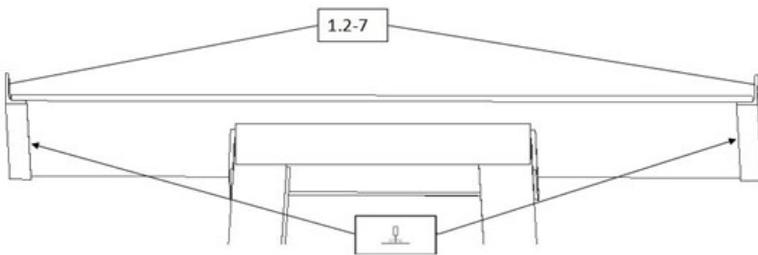
You can stand on the working platform when you want to check or work at the top of the wind pump. To prevent slipping with shoes, angle irons are welded around the perimeter. Their raised edges prevent slipping on the platform.
