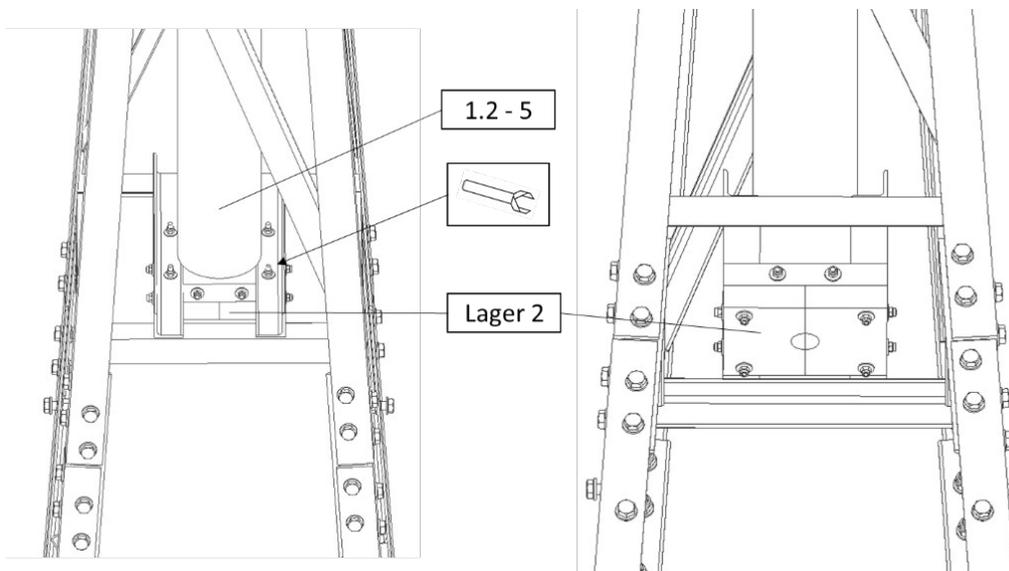
5. Finally, the bearing 2 is screwed to the L-sections at the lower tube end in the mast head [1.2-5].
